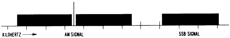
Figure 33. Relative spectrum space occupied by AM signal and SSB signal modulated by frequencies of 200 to 3000 Hz.
