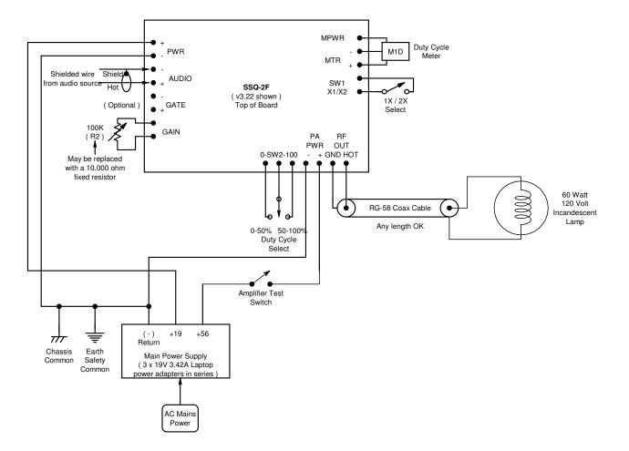
WARNING - You must have a cooling fan set up to blow plenty of cooling air over the heat sink of the IRF730 or the transistor will burn out.
