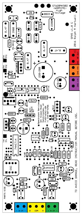
Figure 2 - SPA5 Terminal Block Connections & Component Identification.
