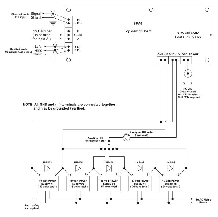
Five power supplies are shown here for a total amplifier DC voltage of 95 volts. More power supplies may be added as required for higher voltages. The maximum DC voltage allowed is 190 volts. The power supply system should be current limited to 3 amperes.
