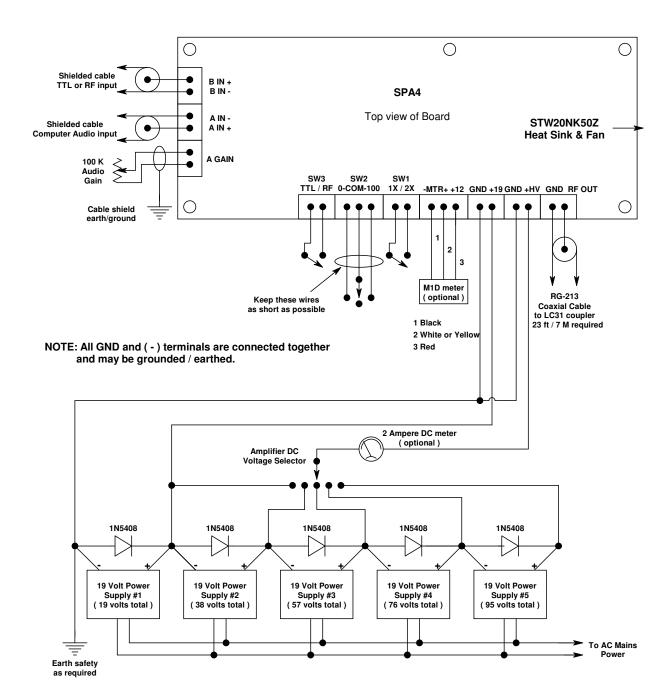
Five power supplies are shown for a total amplifier DC voltage of 95 volts. More power supplies may be added as required for higher voltages. The maximum DC voltage allowed is 190 volts.
