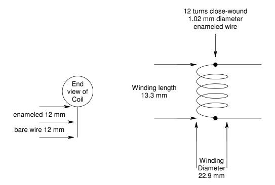
Wire diameter measures 1.12 mm diameter with enamel and 1.02 mm without enamel insulation.
