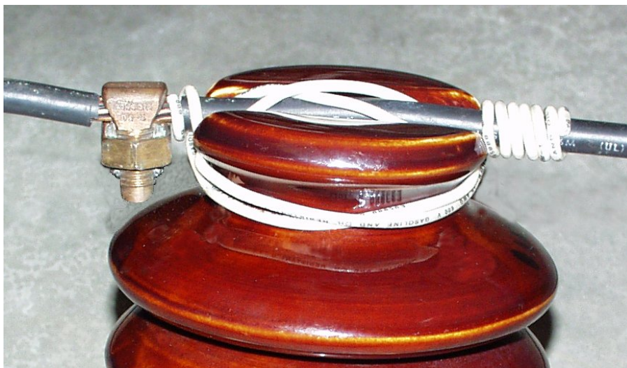
Figure 68 Tie Wire Source Mitigation, Example 1
