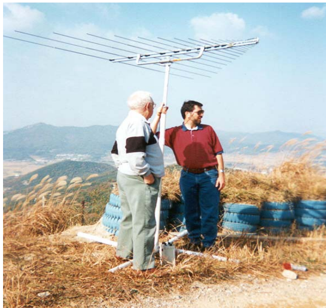
Figure 59 Hilltop Source Location with RFI Locator
