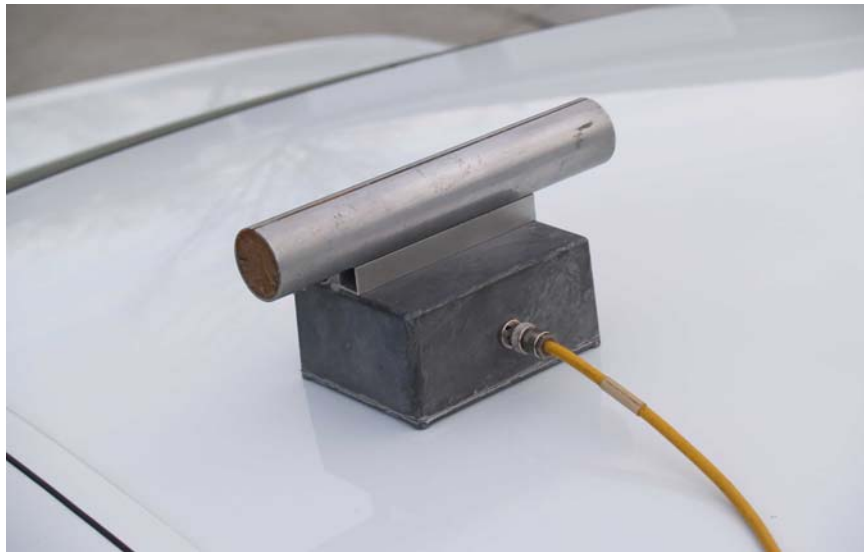
Figure 61 Loopstick Antenna on Roof of Source-Location Automobile
