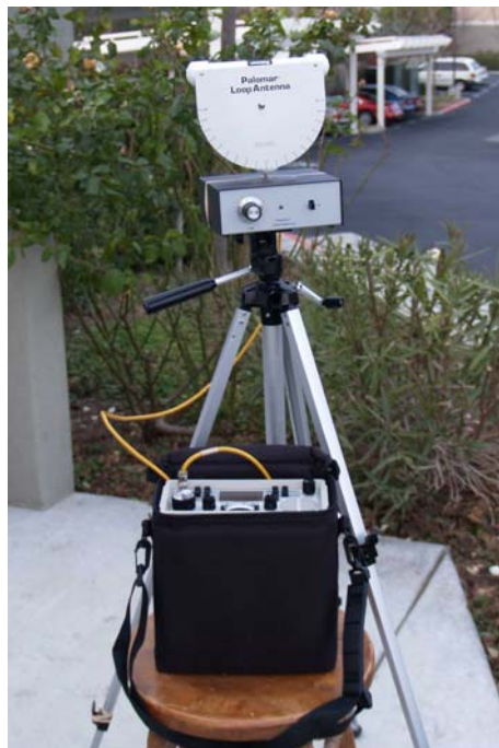
Figure 60 Loopstick Antenna for Location of Power-Conversion Sources
