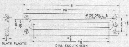
FIG. 12. DIAL ESCUTCHEON is formed \frac{1}{4} -inch thick plastic with window slot for dial scale. It may be painted in a color which matches the color scheme selected for the receiver.
