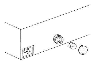
Refer to the figure above. Using a coin, unlatch the cover by turning it slightly counter-clockwise. Remove the battery - a "tool" such as a toothpick may be required to loosen the battery from its mounting. Replace the battery with the negative (button) end inside and the positive (case) end outside. Replace the cover and the radio is now ready to re-program.
