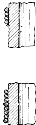
DETAIL NO. 1 TAPE AT START OF WINDING. DETAIL NO. 2 TAPE AT END OF WINDING.
