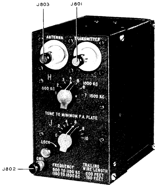
Figure 6-40. Type CU-26/ART-13 Antenna Loading Coil Unit—Front View
