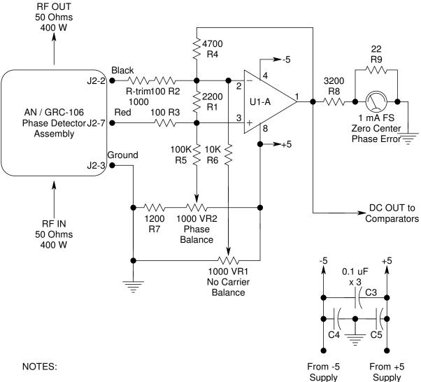
U1 = ECG941, LM158, LM258, LM238, LM2904, MC1458 or equivalent. U1-B Not used.
