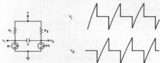
Fig. 2.19. Typical Glow Lamp Astable Multivibrator and Outputs.
